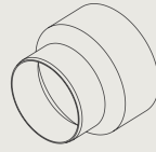
Junction KACL.343 \varnothing 5\ 15/16'' (150) / \varnothing 7\ 7/8'' (200)
